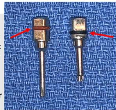
Figure 7: O-Ring Replacement - any implant driver or insertion tool that contains O-Rings should be periodically evaluated for material fatigue and retentive as they may detach from a thumb driver or torque wrench.
